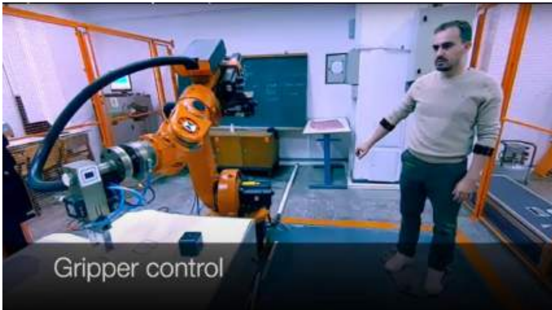
Fig.6. Teleoperation of Kuka KR15
