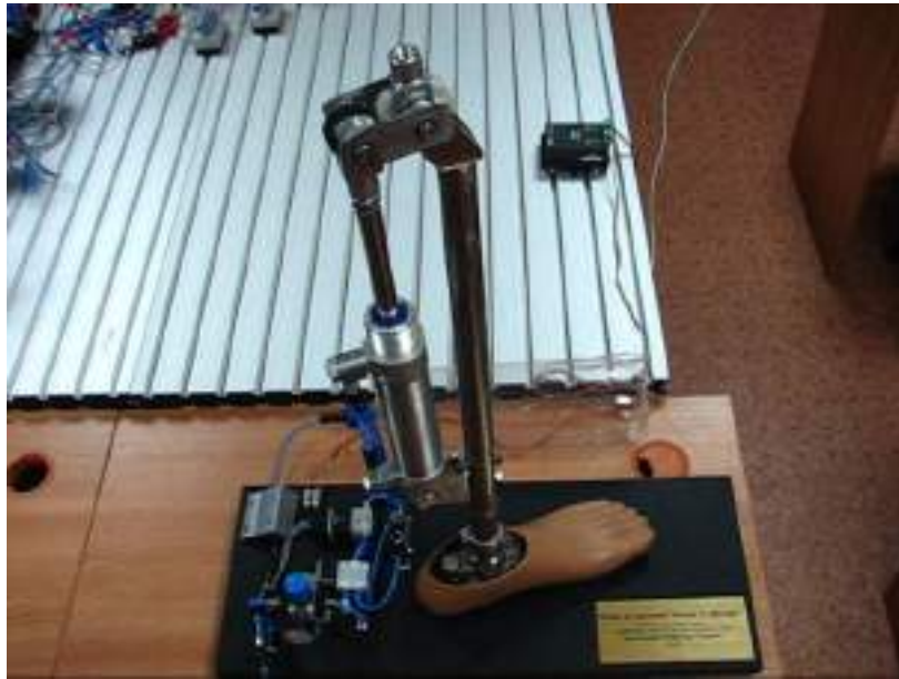
Fig. 13. Experimental prototype of the knee prosthesis
